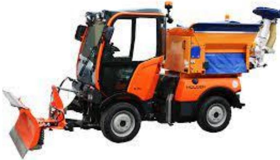
Figure 3 – HOLDER Sidewalk Plow
